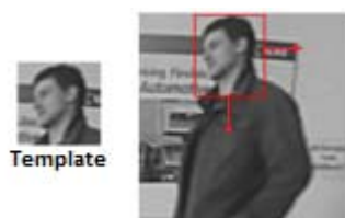
Figure 3: Pattern Matching – Principle Illustration
