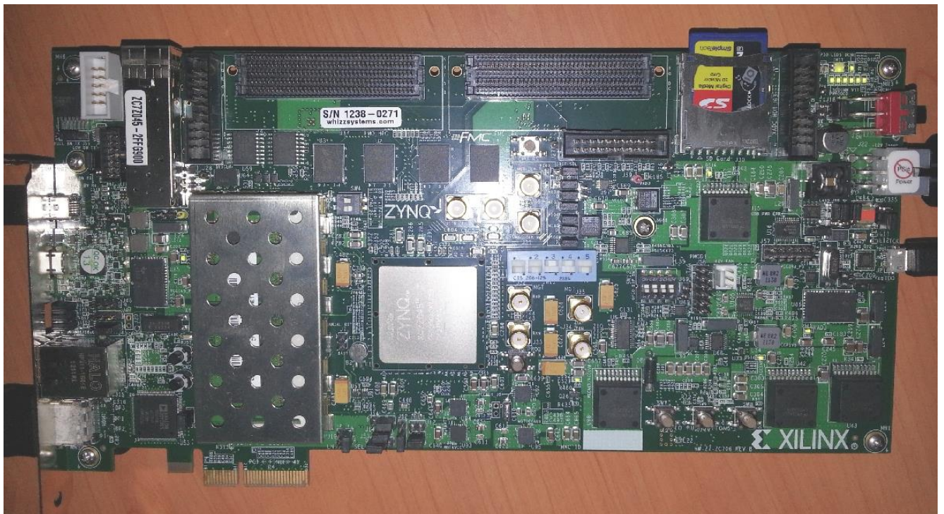
Figure 30: The ZC706 Board (Rev. 1.2) Setup for the logicBRICKS Reference Design
