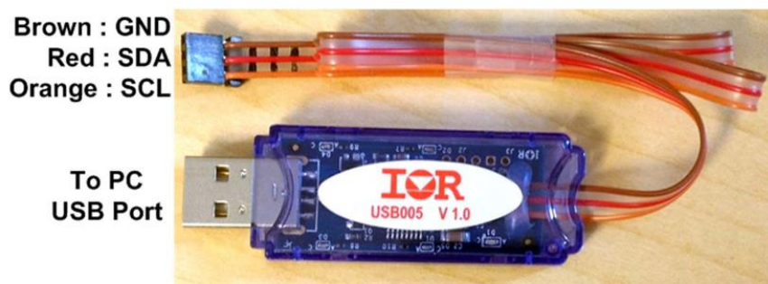
Figure 2.1: Infineon's USB005 Programming Dongle
