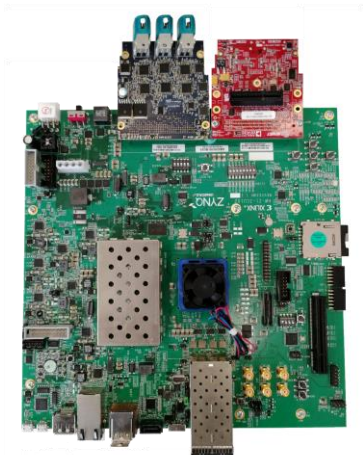
Figure 5: logiVID-ZU-GMSL2 MPSoC Vision Development Kit
