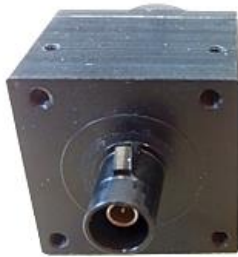
Figure 2: Housing backside with the Rosenberger FAKRA Z TYPE Connector
