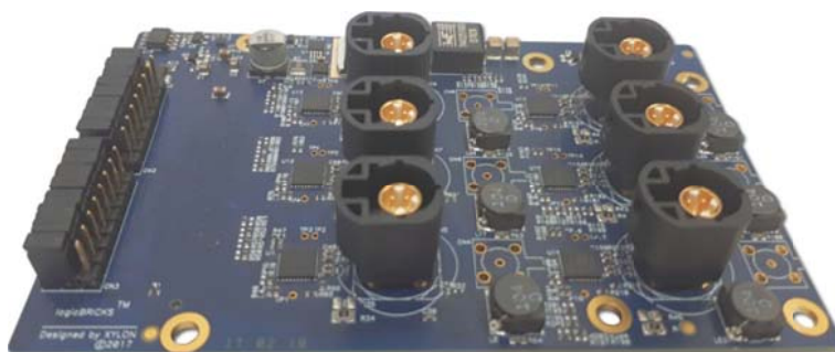
Figure 3: logiFMC-GMSL-96706 Assembled with the RosenbergerHSD Connectors
