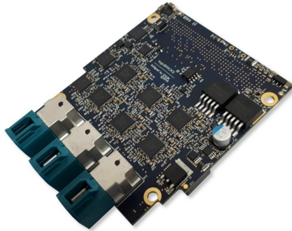
Figure 1: logiFMC-GMSL2 12-Ch GMSL2 FMC Daughter Card
