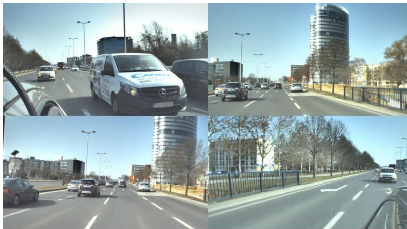
Figure 2: Parallel HDR ISP Processing of 4x 2.3 MP Automotive Cameras by the logiREF-MULTICAM-ISP Reference Design
