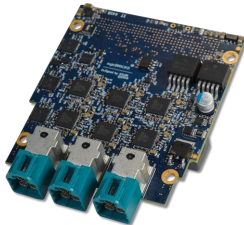
Figure 4: Xylon's logiFMC-GMSL2 deserializer FMC module
