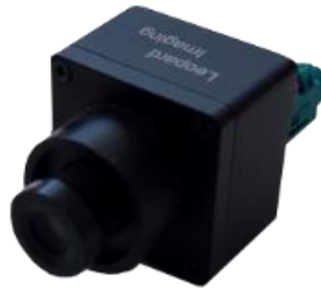
Figure 3: Leopard Imaging LI-IMX424-GMSL2 Video Camera
