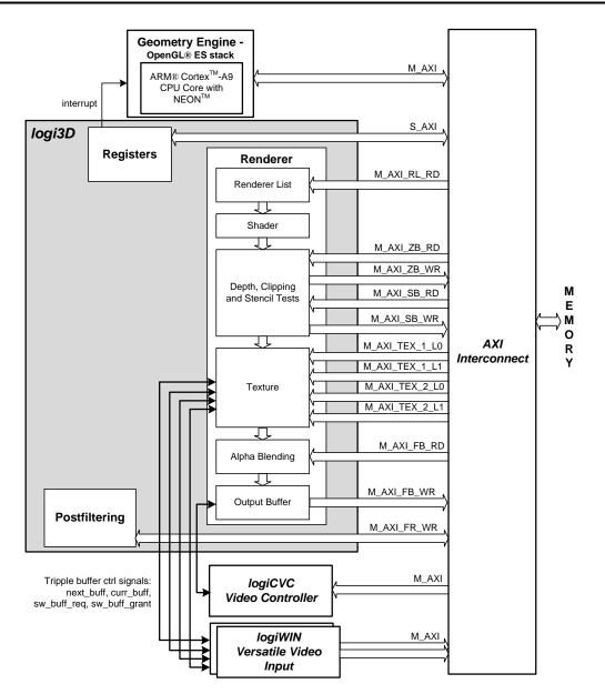
Figure 1: logi3D Architecture (Xilinx Zynq SoC Implementation)
