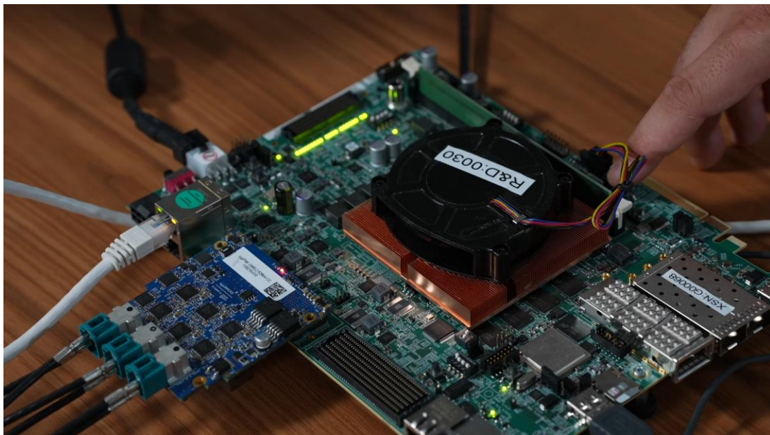
Figure 3: logiVID-ACAP-ISP HDR ISP evaluation kit and VCK190 evaluation kit
