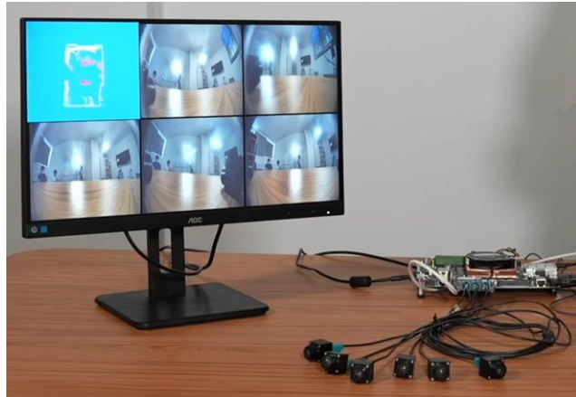
Figure 1: ACAP-VDF Reference Framework provides complete multi-camera to display Versal ACAP designs
