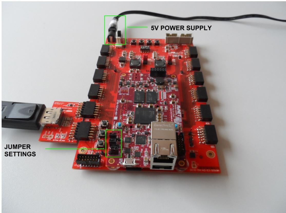
**Figure 6.1 The MicroZed (Rev. B) Setup for the logicBRICKS Reference Design**
