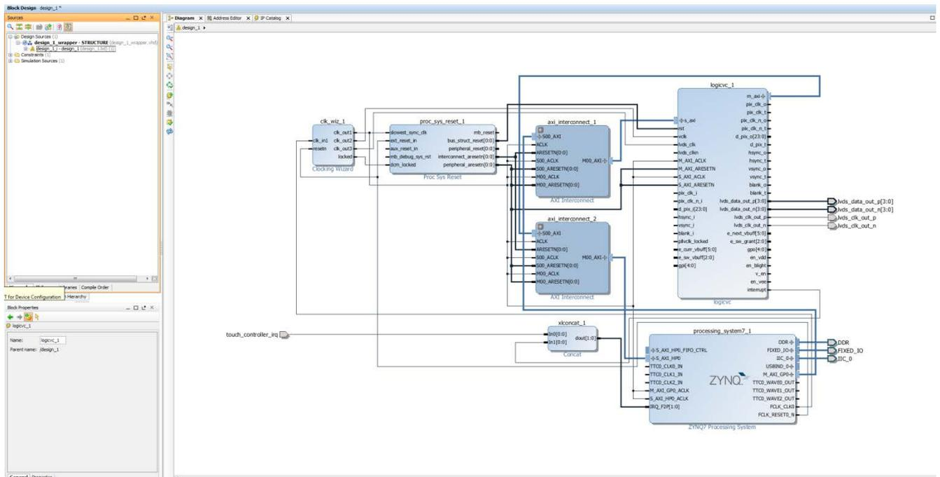
**Figure 4.4 Vivado IP Integrator View – logiREF-DISP-MicroZed project**
