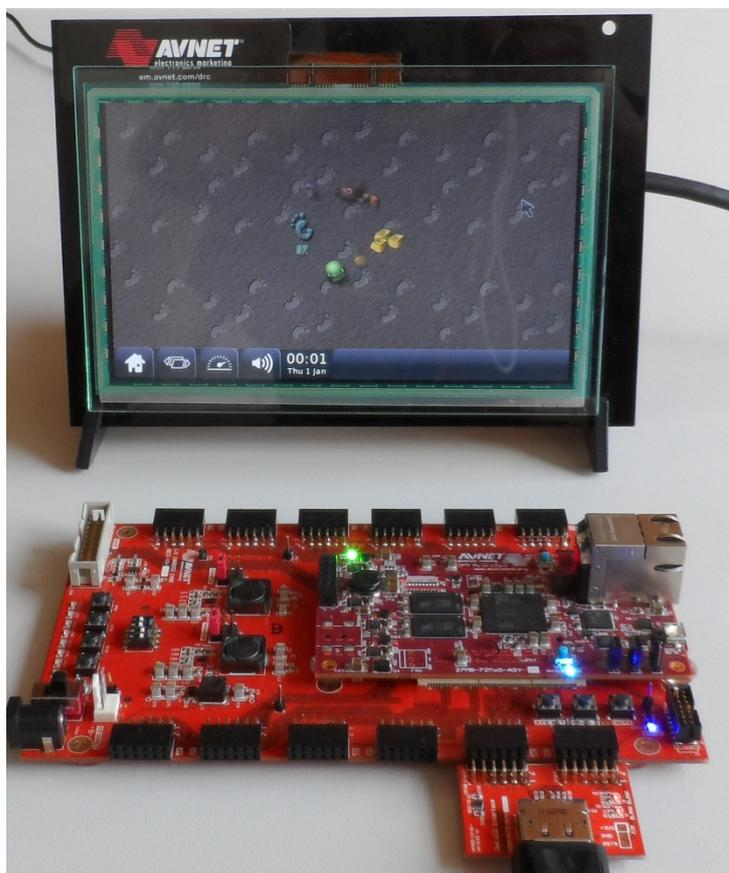
**Figure 1.1 The MicroZed Development Kit Running Xylon's Video Display Demo**
