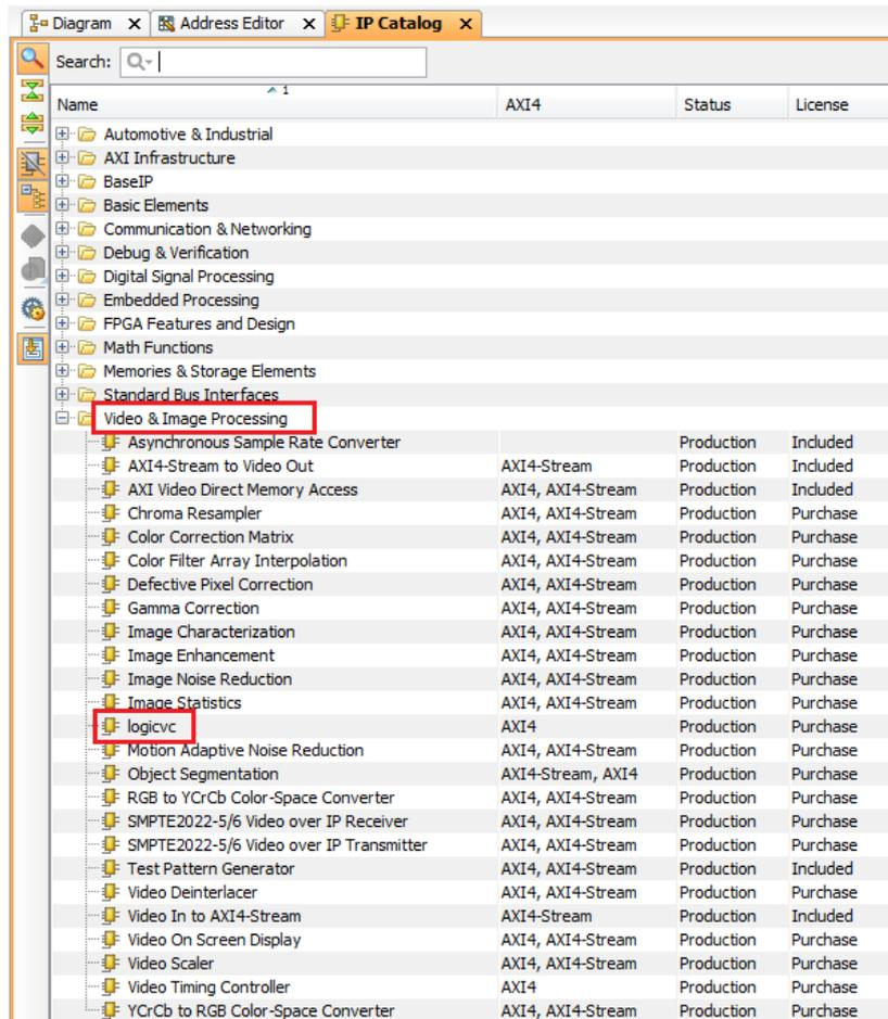
**Figure 2.1 logiCVC-ML IP Core Imported into the Vivado IP Catalog**
