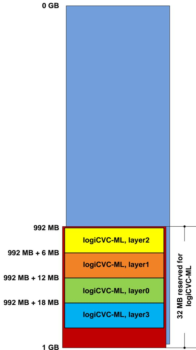
**Figure 4.3 logiREF-DISP-MicroZed Memory Layout**
