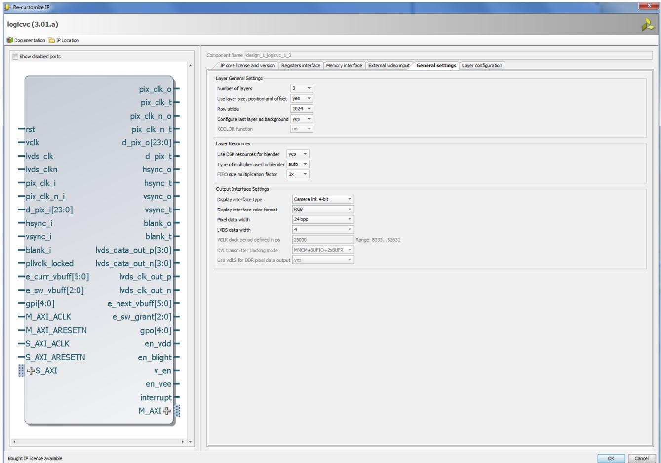
**Figure 2.2 An example of logiCVC-ML IP Configuration GUI**
