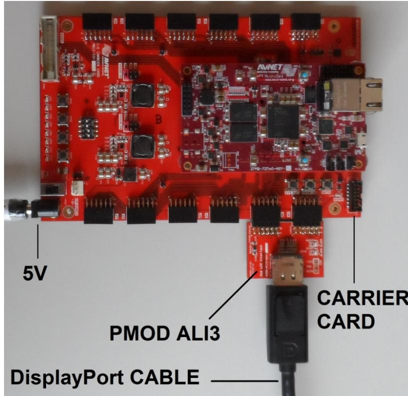
**Figure 6.2 I/O Carrier Module and PMOD-ALI3**
