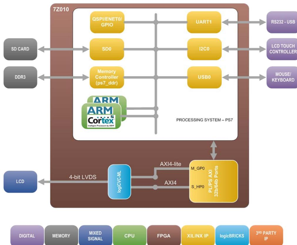
**Figure 4.1 logiREF-DISP-MicroZed Reference Design – Block Diagram**
