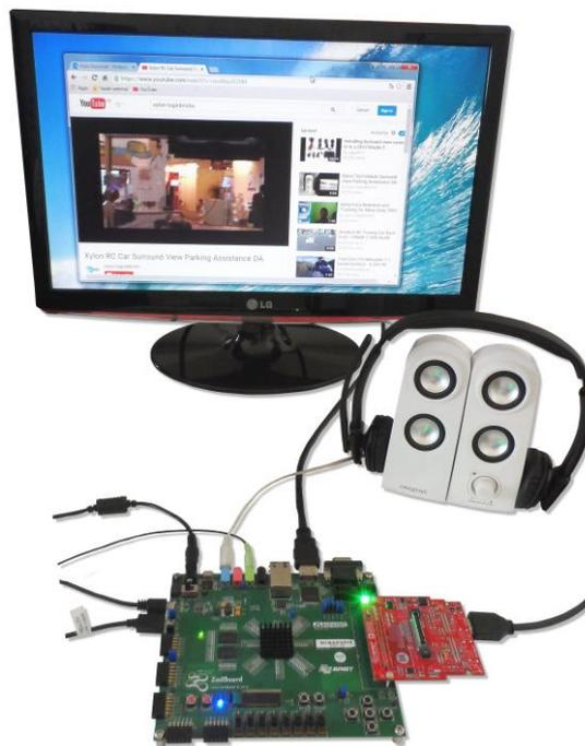
**Figure 1: The ZedBoard Development Kit Running V4L2 Video Capture Demo**
