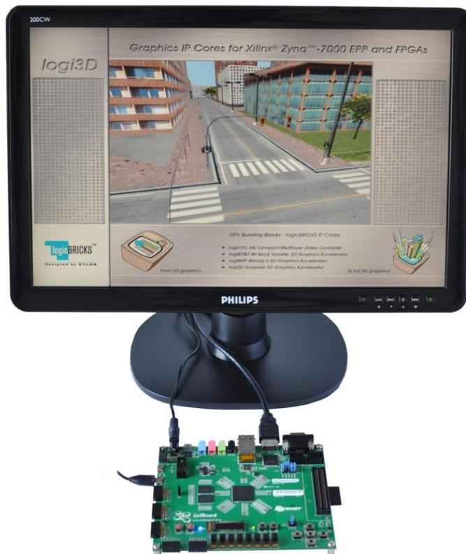
**Figure 1: The ZedBoard Development Kit Running Xylon's 3D Graphics Demo**
