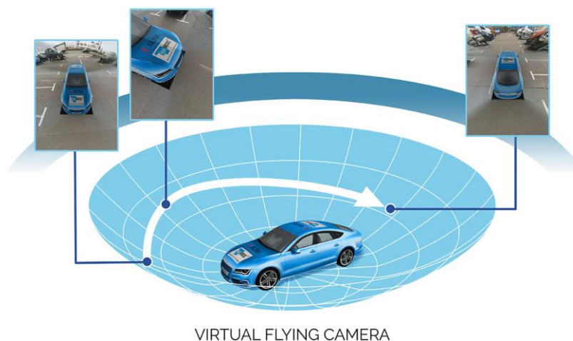
Figure 3: Dynamically changeable 3D views generated by the logiVIEW IP Core
