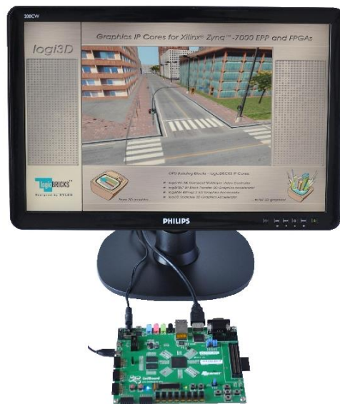
Figure 1: The ZedBoard™ Development Board from Avnet Electronics Marketing Running Xylon's 3D Graphics Demo on Linux OS
